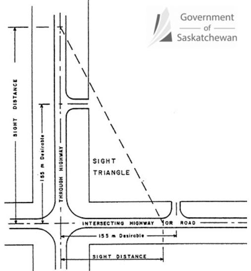
4.18.3 The diagram on the previous page demonstrates the calculation of the sight triangle, where distances "x" and "y" are determined by the Ministry of Highways and Infrastructure depending on the design speed of the through highway and the type of intersecting road:
